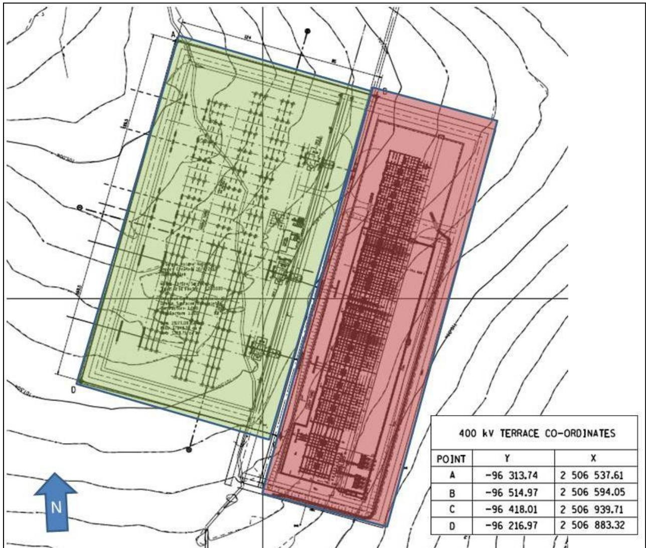
**Figure 10.5:** Proposed Nzhelele Transmission Substation expansion footprint versus the approved Bokmakirie Distribution Substation expansion footprint
